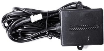
后方来车预警雷达 Early-warning radar for incoming car from behind
