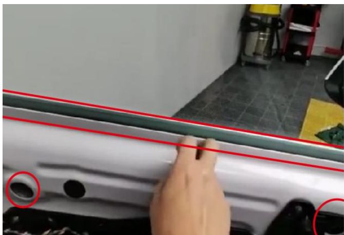
3. 拿出标示处胶条和胶塞把玻璃螺丝对上孔位 Take out the adhesive strip and the stopper at the marked area. Align the glass screw to with the hole.
