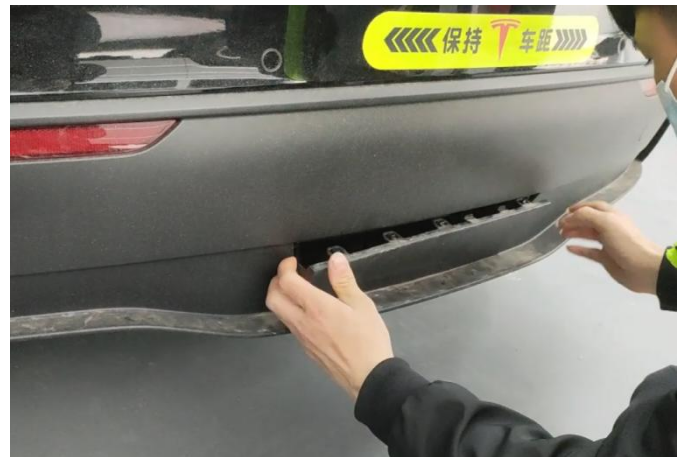
4. 拆下车尾盖板 Take off the tailgate cover
