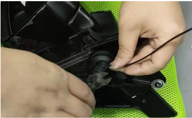
11. 用扎带扎住防水胶塞 Tight the waterproof with the ribbon
