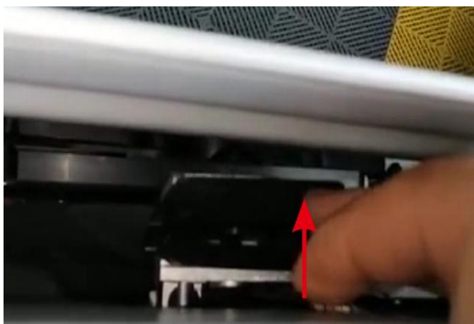
5. 玻璃槽卡扣需要同时用螺丝刀拨开取出玻璃 the slot buckle of the glass need to be opened and removed at the same time.
