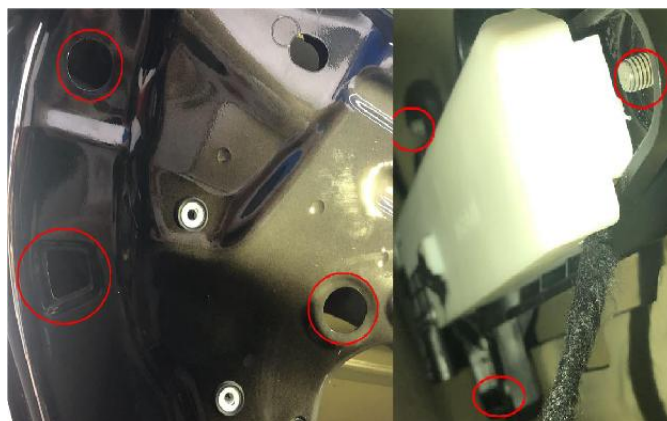
8. 取出上图三颗螺丝，拆下原车把手 Remove these three screws and take off the original handle.
