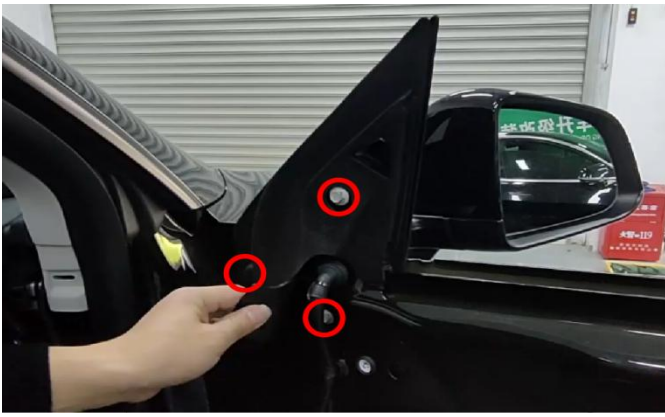
1. 卸下三颗螺丝拿出后视镜 Unscrew these three screws, and take out the rearview mirror
