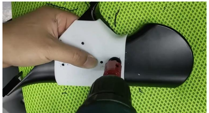
6. 用我司模块照模打三小一大四个孔 Punch four holes using our module to mold. (Three small holes, one large hole)
