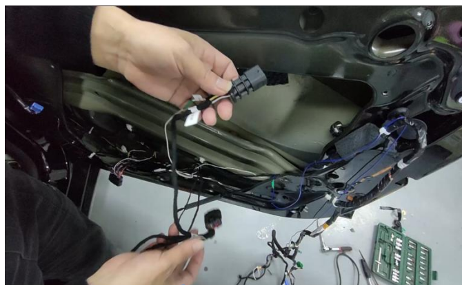
2. 插头与原车锁头拔出的母座对插 Connect our plug to the socket which unplug from the original lock.
