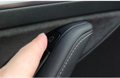
内拉把手开关门 Open/close the door by Interior handle
