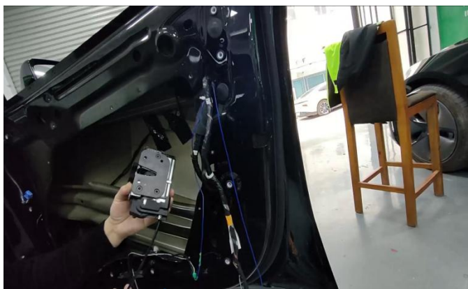
1. 替换原车锁头，用我司螺丝固定 Replace the original lock, fixed with our screws.
