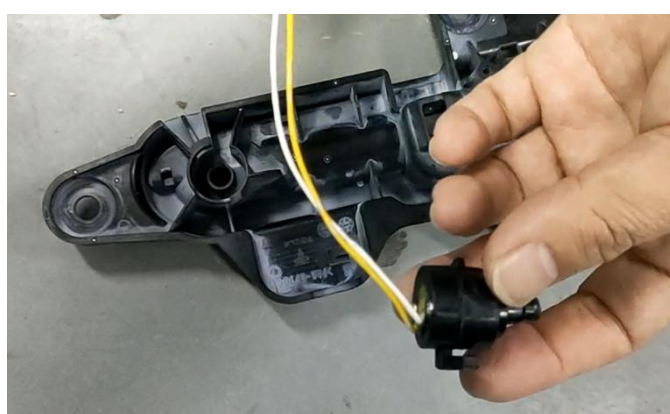
4. 下压旋转取出原车按钮替换我司按钮 Press and rotate to remove the original button, and install our button
