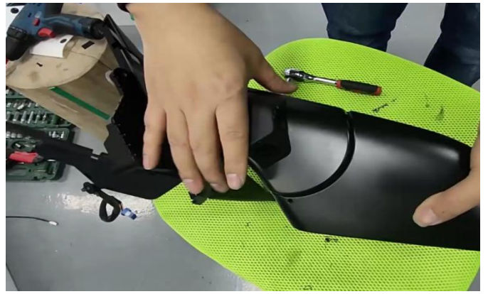
10. 把拆下来的盖板扣回去，然后恢复胶条打紧螺丝 Recover it, and fixed.
