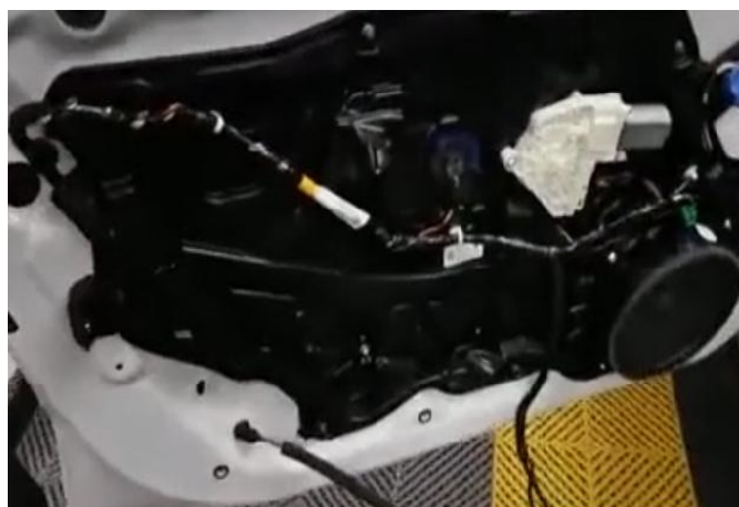
6. 拔掉与饰板相连的插头 unplug the wire on the trim panel.
