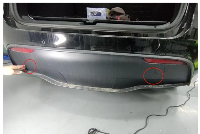
6. 根据智能门安装位置安装对应的左右车尾雷达 install the radar to the position as the figure shown.
