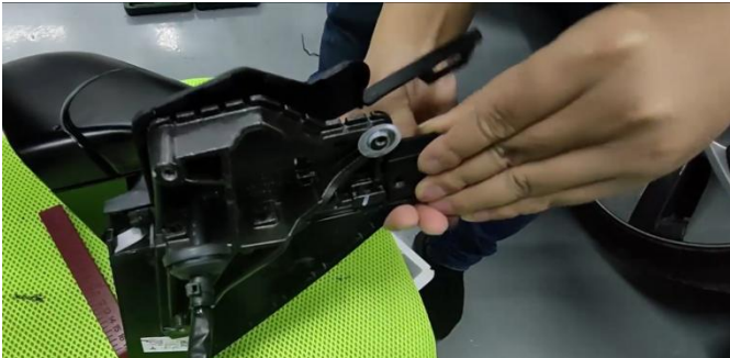
3. 拿下胶条 remove the seal
