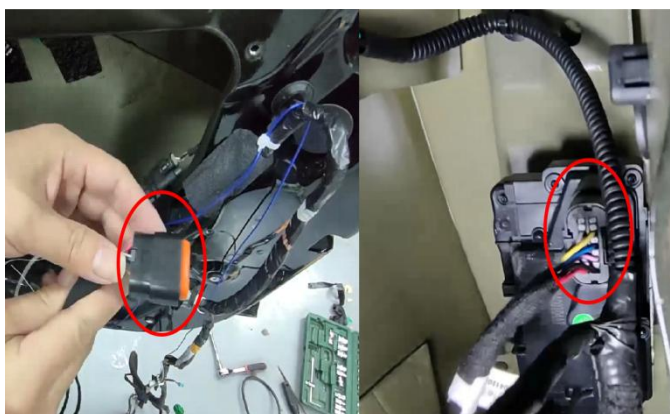
3. 与电吸锁头直接对插 Connect to the electric lock
