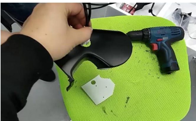
7. 把雷达线穿过大孔 Thread the radar wire through the big hole.
