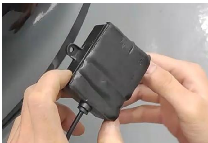
5. 不要把 3M 胶贴到下方了，不然会导致雷达不灵敏 Don't paste the 3m sticker under the radar, or it will not sensitive.
