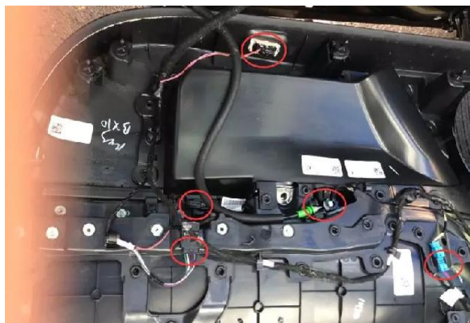
4. 把与盖板相连的插线拔下拿下盖板 Unplug the wire and take out the trim panel.
