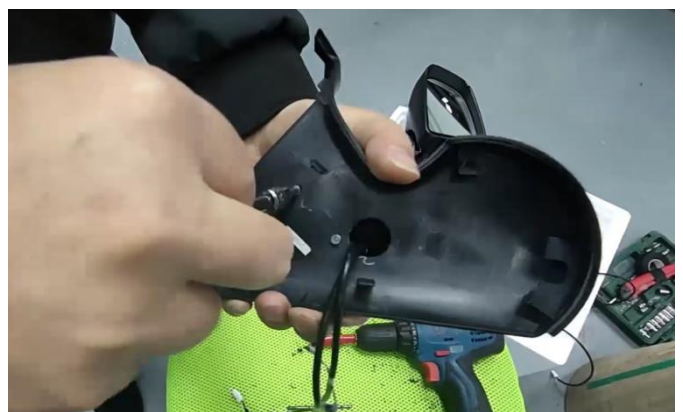
8. 三个小孔用我司螺丝固定雷达 fix the radar with our screws.
