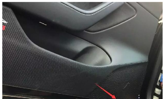
2. 用撬刀撬右下角卸下门饰板 Pry the lower right corner to remove the door trim panel
