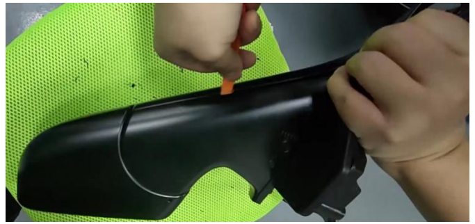
4. 用撬刀沿着缝隙撬开 pry open along the gap
