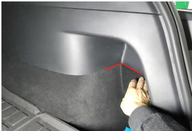
3. 雷达线材从车门穿过波纹管到尾箱通风口到上图走线，再穿到雷达安装对应的位置 The radar wire pass through the corrugated pipe from the door to the tailgate vent.and go into the install position.
