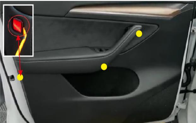
1. 卸下上图三处螺丝 Remove the screws shown in the figure above
