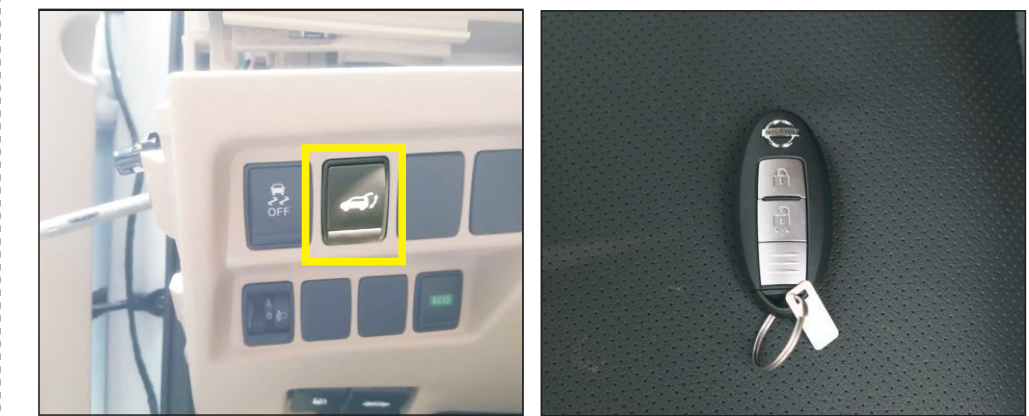
Press the front switch button to open/close the tailgate
