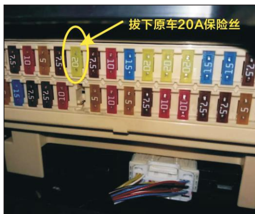
7. Remove the trim at the bottom of the main drive, remove the original car 20 a fuse, plug in our power plug
