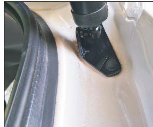
3. The original car right bracket will be removed, replaced our lower bracket (ball head outwards), with the original screw fixation
