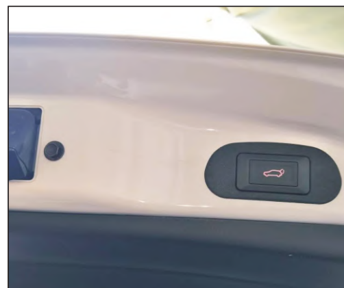
15. Install the tail door switch to the position as shown
