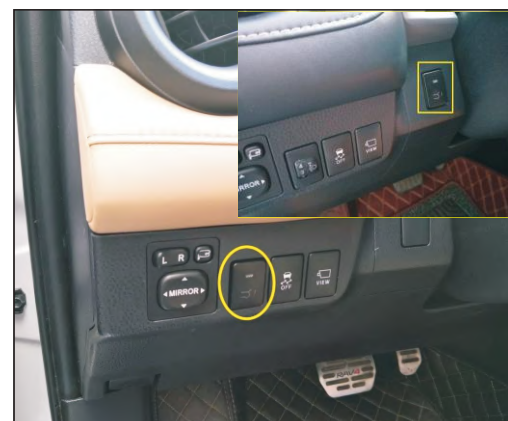
9. Main drive to remove the original empty button, the installation before we switch button (choose one)
