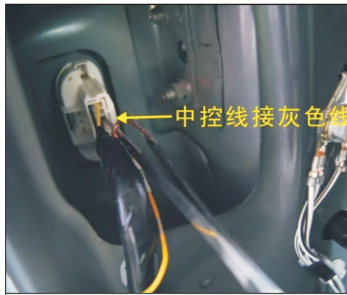
11. Central Line by gray line (from left to right the second ranked the third hole)
