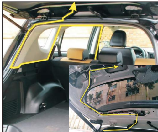
13. And the power cord, switch before the Central Line through the rubber plug walked to the central control box
