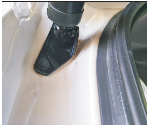
2. The original car bottom bracket will be removed, replace our bottom bracket (ball head outwards), with the original screw fixation
