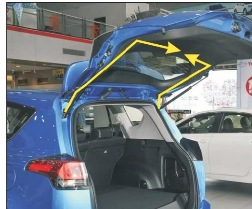
6. Hall walk line after line through the hole to end door cover plate
