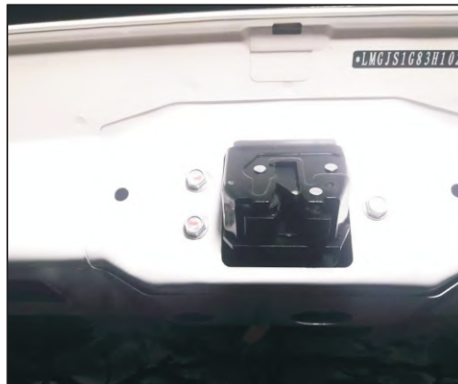
14. Abort the original screw, remove the original car lock, installed on our electric absorption, use the original car screws
