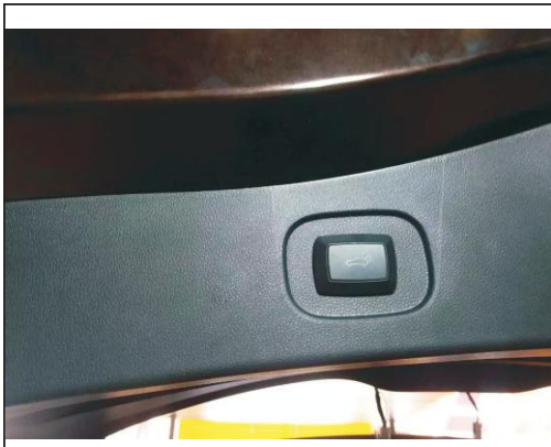
19. In the original car trim punch installed our door switch button
