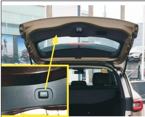
16. In the tail door trim punch, install door switch our end
