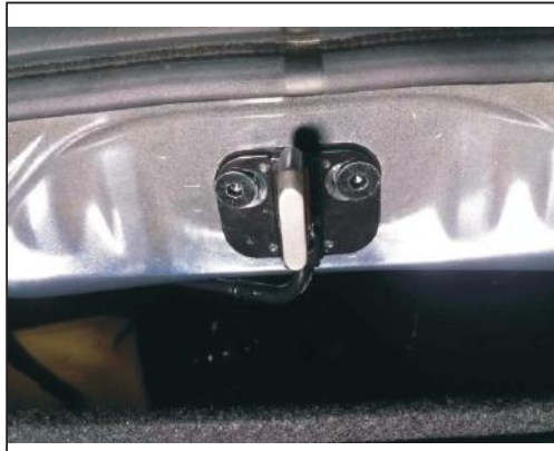
17. Remove the original lock buckle, install our electric lock
