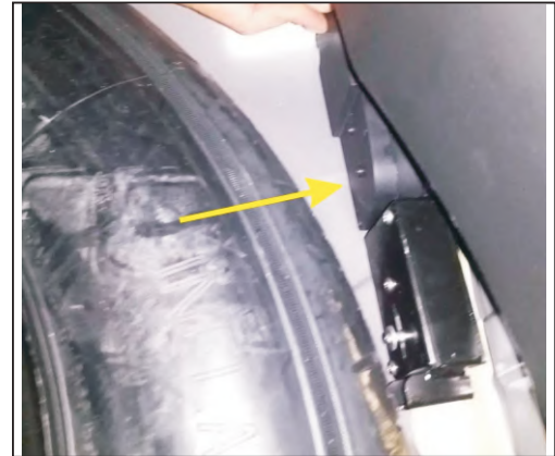
18. The motor installed in a spare tire, with our company 3 m glue
