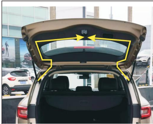
8. Hall line through the rubber plug door trim line to end
