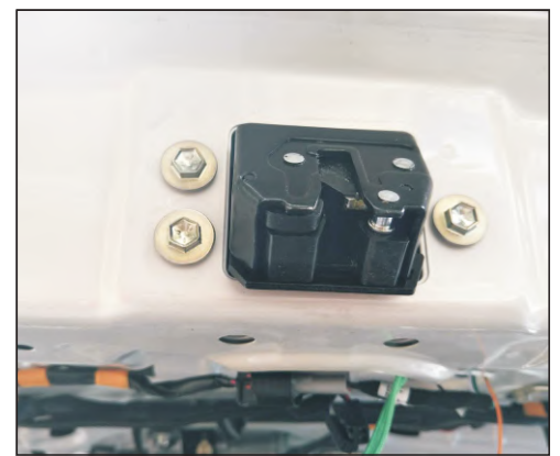
24. Remove the original door lock, install our company on the electric suction, use the original car screws
