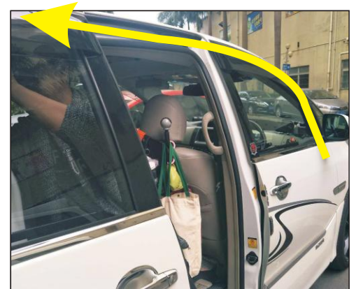
23. Before the main driving switch line is along the yellow line arrow to the tailgate cover
