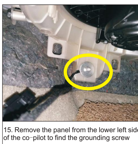
15. Remove the panel from the lower left side of the co-pilot to find the grounding screw
