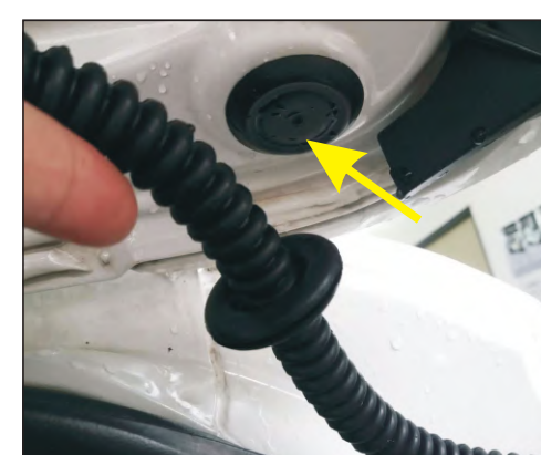
8. Remove the original rubber plug from the left strut, and let the Hall wire pass through the reserved hole.
