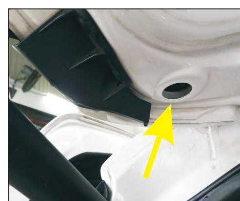
7. Remove the original rubber stopper from the right strut. The Hall wire passes through this reserved hole.
