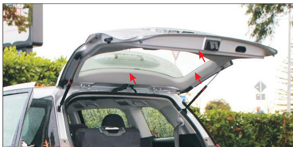
1. As shown in the figure, remove the plaque and the original car strut
