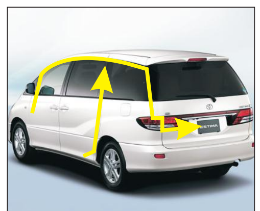
22. The co-pilot's power line and center line are routed from the top of the vehicle along the yellow arrow to the tailgate cover
