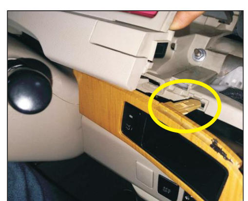
20. Remove this trim plate to facilitate the installation of the front switch button
