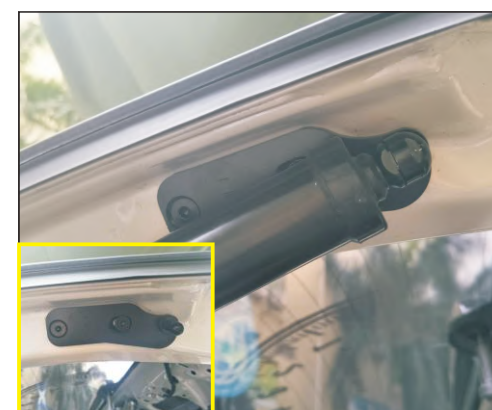
2. Remove the left upper bracket of the car, install the upper right bracket (ball head outwards), and fix it with our screws
