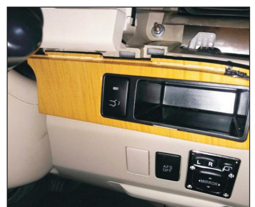
21. Remove the original car button, install our special front switch button
