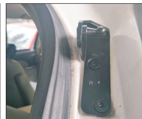
5. Remove the lower right bracket of the original car, install the lower right bracket of the company (ball body facing outward), and fix it with our screws
