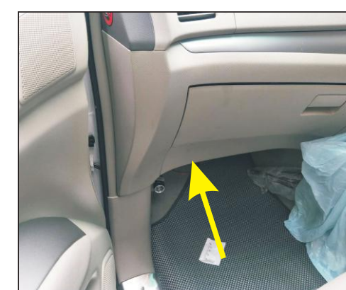
12. Remove the plaque under the co-pilot to find the original car power
