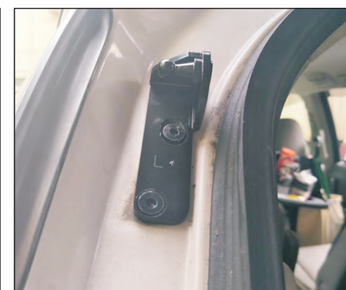
3. Remove the left lower bracket of the original car, install the left lower bracket of the company (ball body outwards) and fix it with our screws
