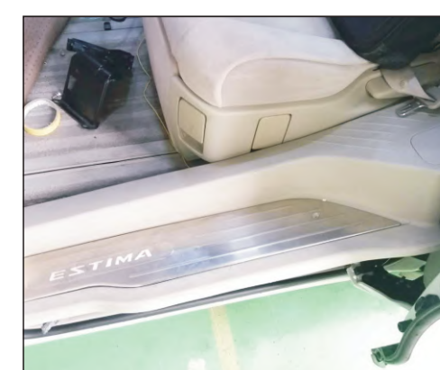
16. Remove the plaque at the second door pedal of the first officer
