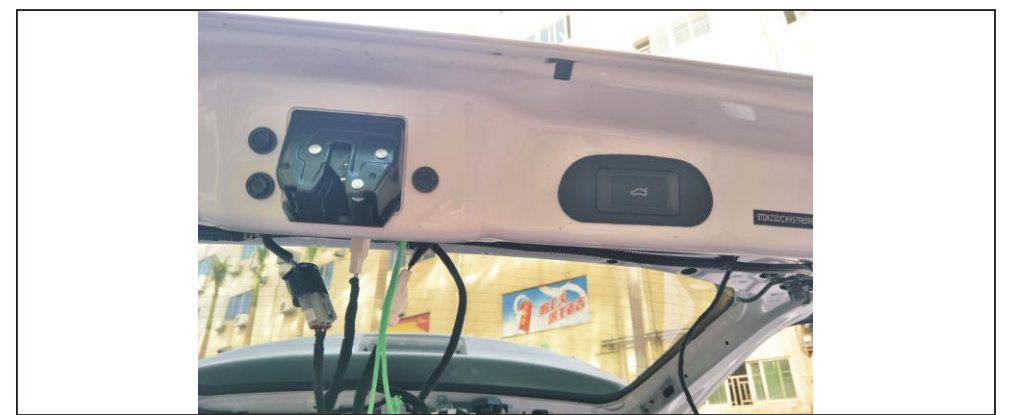
Tail door height setting Raise the tailgate to the ideal height, press the tailgate to install the switch button, 3-5 seconds will appear "beep" sound, release the handle, press the tailgate again, The key is off, the tailgate is closed, and then there are two "squeaks", that is, the tailgate is completed.
