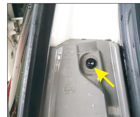
11. Install our flat head screws (same as left and right steps)
