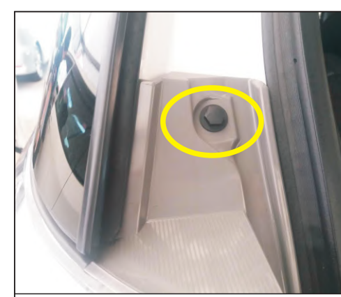
10. Detach the screw in the tailgate flow sink (left and right steps)
