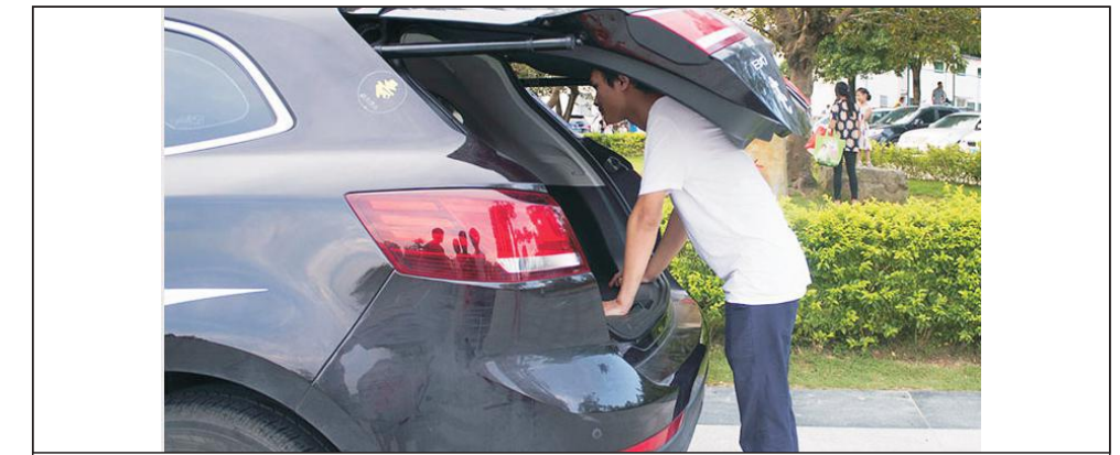
Anti-pinch function: 1. Anti-clamping: When the obstacle is under the tailgate closed, when the tailgate is closed, when you encounter an obstacle, you will bounce back in the opposite direction 2. Door collision avoidance: When the obstacle is behind the tailgate Obstacles will bounce back in the opposite direction
