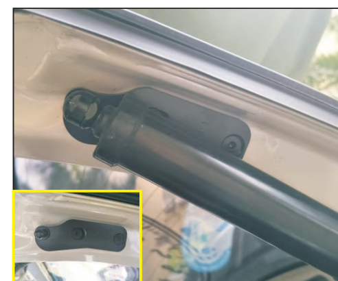
4. Remove the upper right bracket of the original car, install the upper right bracket of the company (ball head outwards), and fix it with our screws
