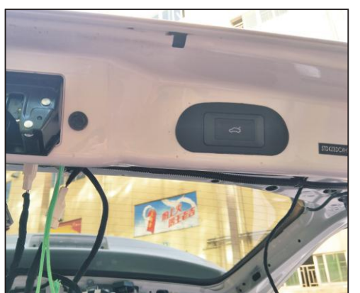
33. Remove the trim plate and install the end button of our company. The rear door socket and the socket of the three-way wiring harness
