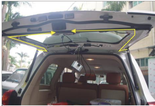
2. Remove the trim panels, the Hall wire is routed to the tailgate trim board
