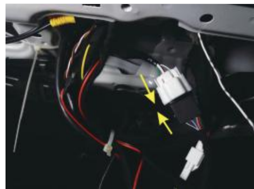
12. Connecting three-way connection socket At the tailgate trim panel, find this socket and pull it out, then plug in our three-way adapter
