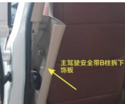
7. Remove the trim board from the B-pillar of the driver compartment seat belt
