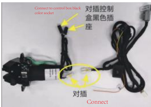
8. Central control wire connect with red and white color wire
