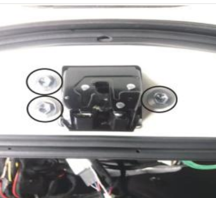
10. Install specially designed electric suction lock and fix it with original screw
