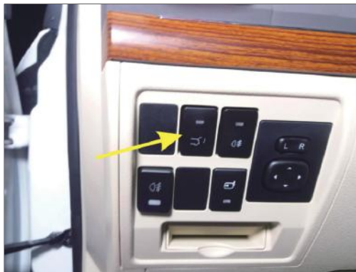
5. At the driver compartment finds the corresponding switch position according to the picture, and replaces the spare part with a dedicated switch.
