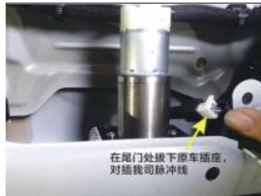
6. Pull out this socket at the tailgate and insert our pulse wire.
