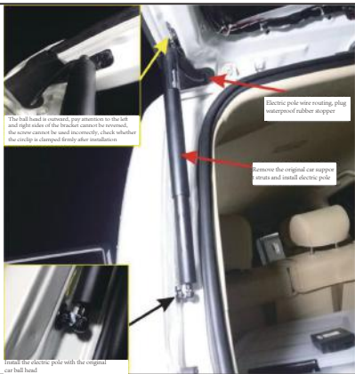
1. Remove the original support struts and brackets, install our specially designed bracket and electric pole, the electric pole wire runs from the top (left and right steps are the same)
