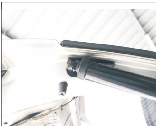
1. Remove the original car bracket, installation of upper bracket and brace, use our screws (or steps)
