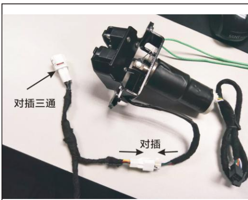
7. The electric socket absorption and tee harness to plug from the socket
