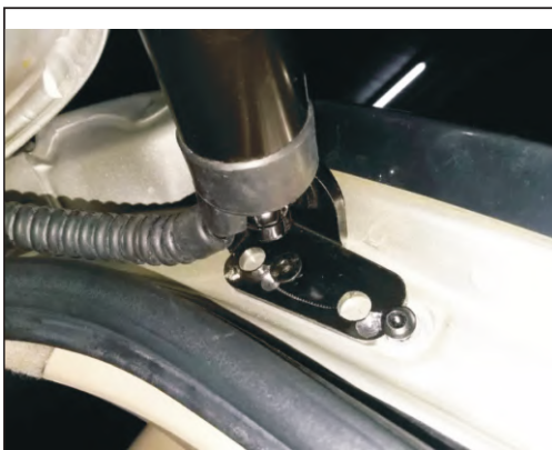
2. Remove the original car right bracket, installation bracket at the lower right, with our screws
