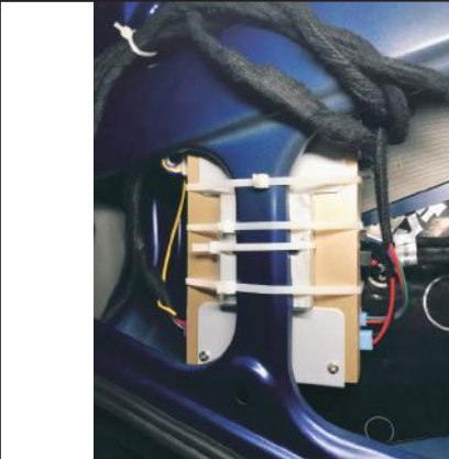
16. Installation position and control box, with our cable tie
